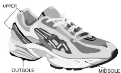
**UPPER** – the soft body of the shoe made of materials ranging from lightweight mesh to heavier leather. Upper materials provide some of the stability comfort of the shoe. The heel counter (reinforced, inflexible cup) is built into the upper of running shoes to surround the heel and pad the Achilles tendon; heel counters come in varying degrees of stiffness. A stiffer heel counter will promote rearfoot stability to help control pronation.
